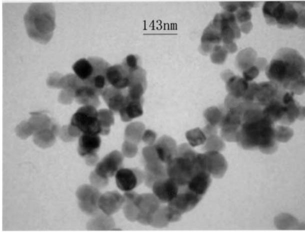
Figure 1 Transmission electron microscope (TEM) micrograph of nano-sized precipitated calcium carbonate synthesized by high gravity method.
