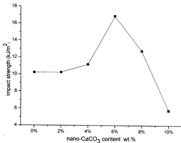
Figure 2 Impact strength of EP composite filled with nano-CaCO<sub>3</sub>.
